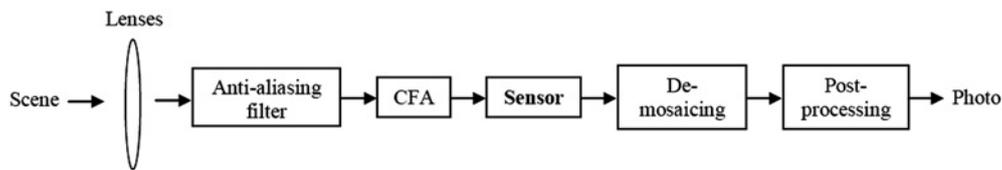
Fig. 1 Process of image acquisition that takes place in a typical digital camera
