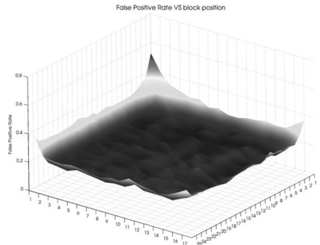
**Fig. 6** EXP\_512: false-positive rate as a function of the position at which the SPN block is extracted, with respect to a  $17 \times 25$  regular grid, and blocks of  $512 \times 512$  pixels
