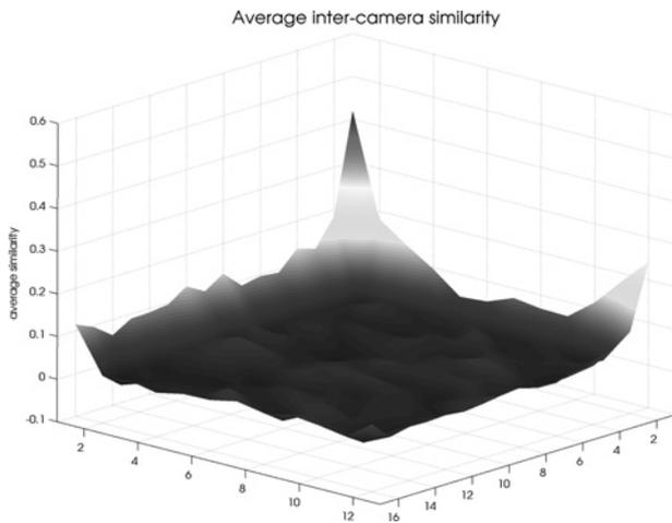
**Fig. 5** Average inter-camera similarity, measured in terms of normalised cross-correlation, of the SPN, as a function of the SPN block position
