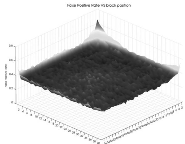
**Fig. 7** EXP\_256: false-positive rate as a function of the position at which the SPN block is extracted, with respect to a  $41 \times 57$  regular grid, and blocks of  $256 \times 256$  pixels
